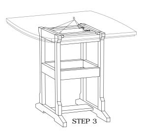
Attach Table Top to base using uncolored screws (B). From the underside screw through pre-drilled holes in the aluminum frame into base assembly.
